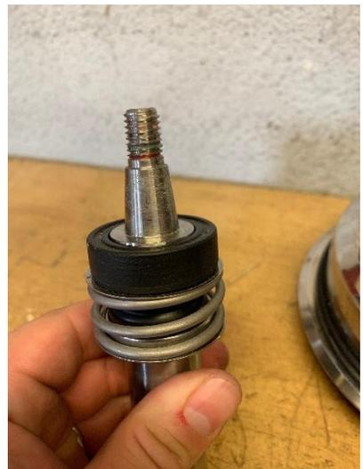
8. With the Carbon seal and gasket (lower mechanical seal) place it at the bottom of the groove inside of the pump cover, gasket side down. It is important to have the carbon side facing UP!
