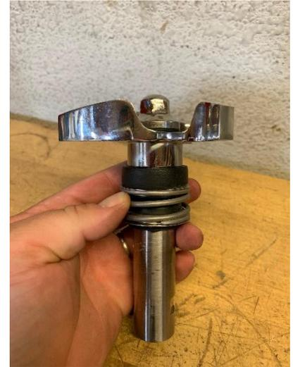
6. Once both pieces are free, you may take off the old mechanical seal (the gasket with spring) and replace it with the new one. Be sure to face the carbon side DOWN and the large rubber side UP! (see right)
