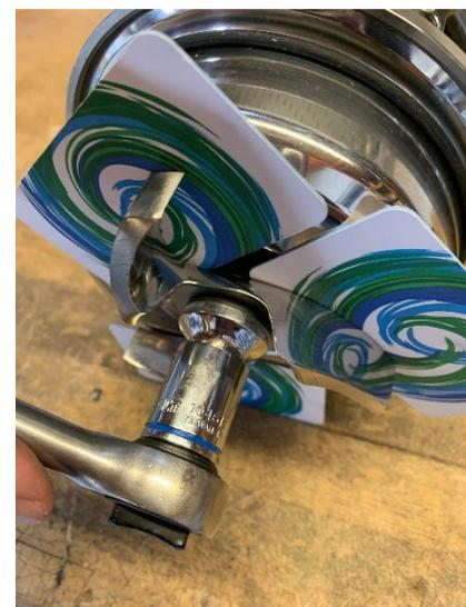
19. If you would like to, you can confirm your spacing is correct with a caliper. The proper spacing should be between 0.3-0.5mm between the back of the impeller to the pump cover.
