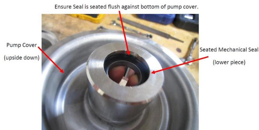
11. Push the pump cover back into place, then slide the impeller shaft over the motor shaft, lining up the lock nuts grooves.
