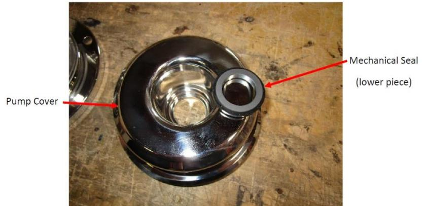
9. Using a pipe, such as PVC, push down on the lower mechanical seal to get an even distribution of pressure to fit inside of the lower groove. Be sure to not to press too hard or hit with a hammer or mallet as the carbon can crack or break if too much pressure is applied.
