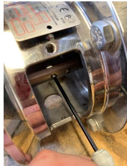
17. Once the set screws are tightened down the impeller blades should be mostly set in place. Tighten down the cap nut with the 16mm socket, securing the placement of the impeller blades, while having a wrench on the shaft to hold the shaft in place.
