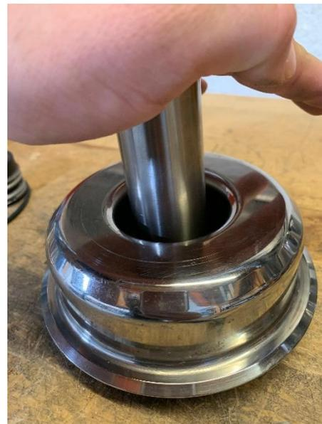
10. Ensure there is a good and even seal between the stainless steel and the lower mechanical seal (as seen on right)
