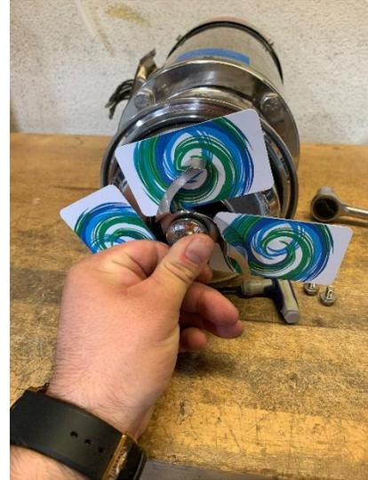
16. While pushing against the cap nut to maintain proper spacing, tighten down the two lock nut screws on the impeller shaft. You may want to add blue Loctite to the screws before placing them to lower the likelihood of loosening
